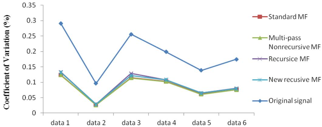
Figure 8. Performance comparison of new recursive median filtering scheme with other variants of median filters
