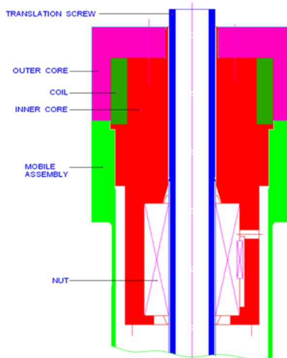
Figure 2. Electromagnet of CSRDM
