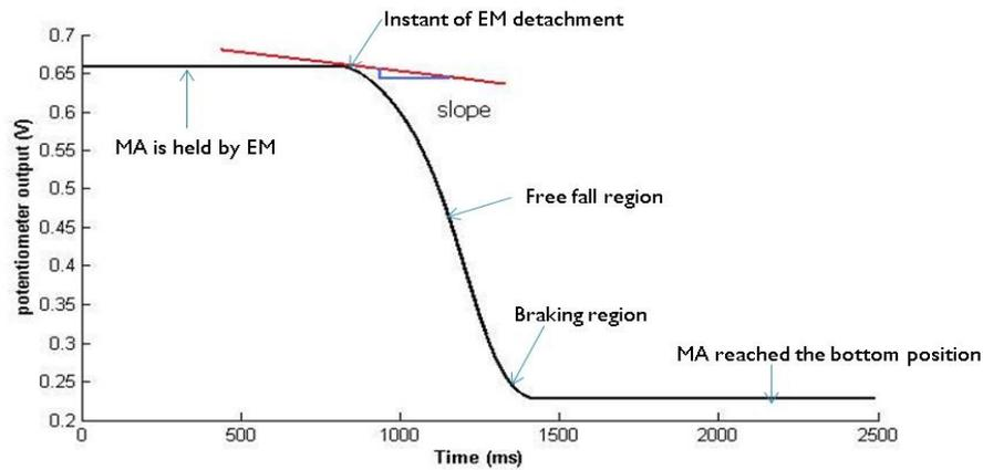
Figure 5. Ideal Displacement vs. time curve during SCRAM
