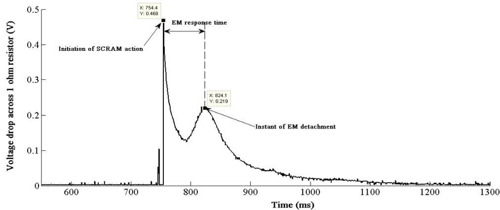
Figure 4. A typical EM response curve (taken for a drop height of 1085 mm)
