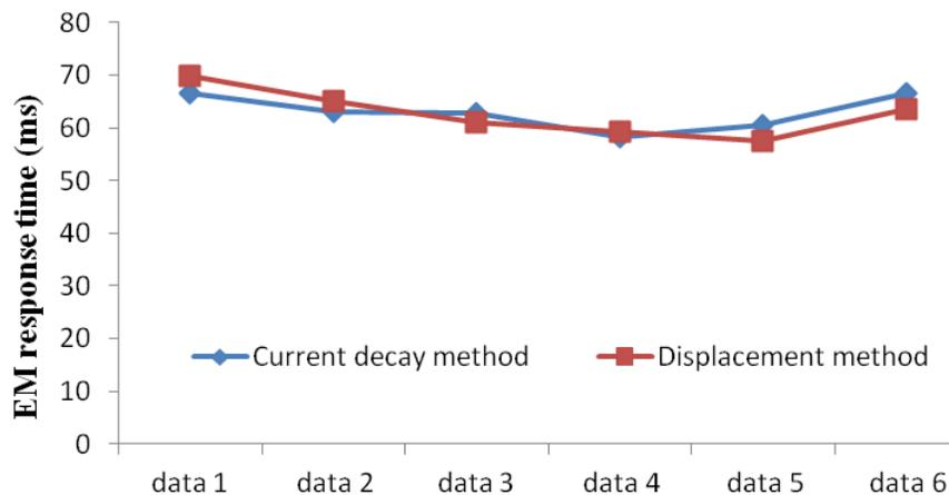
Figure 10. Comparison of results of displacement method with current decay method
