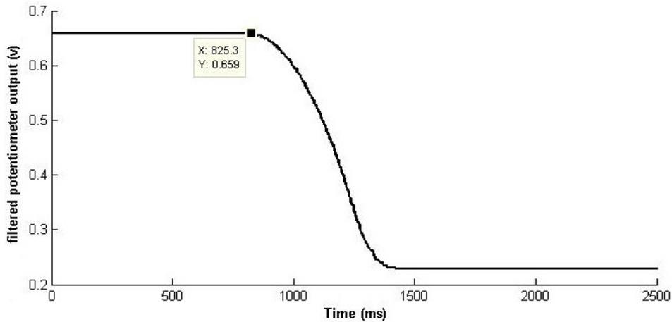
Figure 9. Displacement vs. time curve from potentiometer signal filtered by proposed filter
