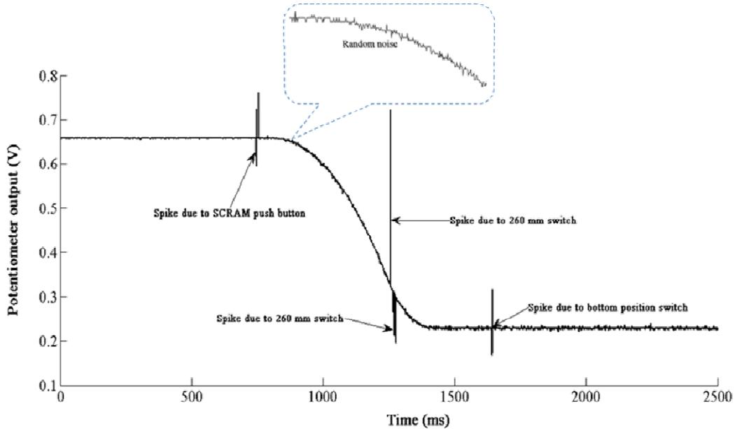
Figure 7. A typical Displacement vs. time curve
