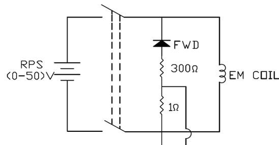
Figure 3. Energising and de-energising circuit of EM
