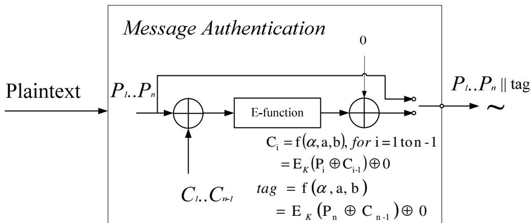
Figure 6. Cipher Block Chaining Message Authentication Code.
