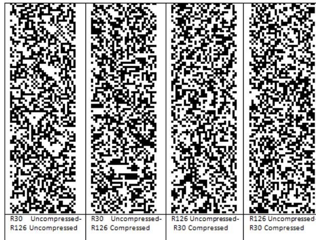
Figure 8. Space-Time diagrams for Rules 30 and 126
