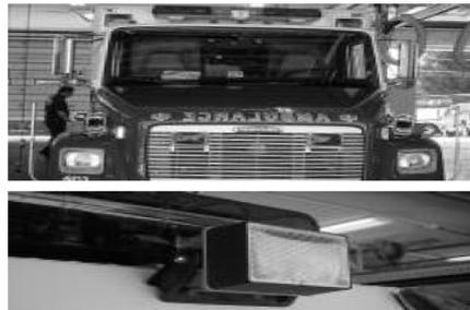
Figure 2. Light-based emitters installed on an Ambulance.
