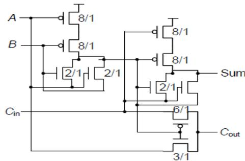
**Fig. . 3.** SERF full adder design
