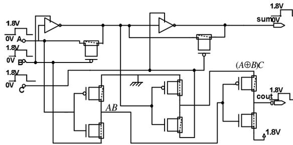
**Fig. .9.** proposed 12T full adder design
