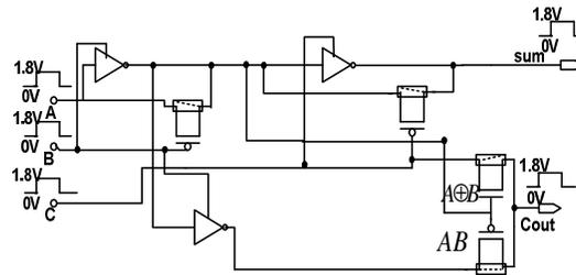
**Fig. 10.** proposed 10T full adder design
