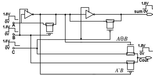
**Fig 11.** Proposed 8T full adder design
