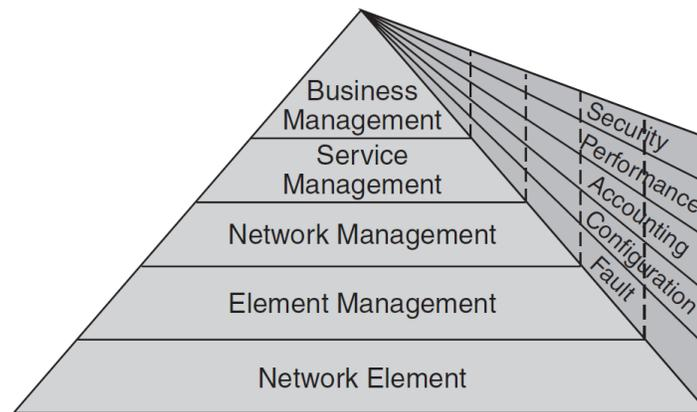
Figure 1 TMN Reference Model Refined with FCAPS<sup>8</sup>
