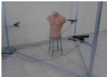
Figure 2. Placing the mechanism of 3d cameras and object to be modelled
