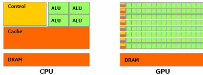
Figure 1. CPU and GPU architecture [18].
