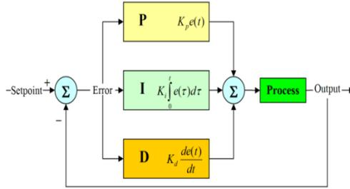
Figure 5 PID controller applied to the nonlinear plant
