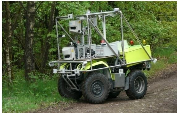
Figure 1 AMOR autonomous mobile robot
