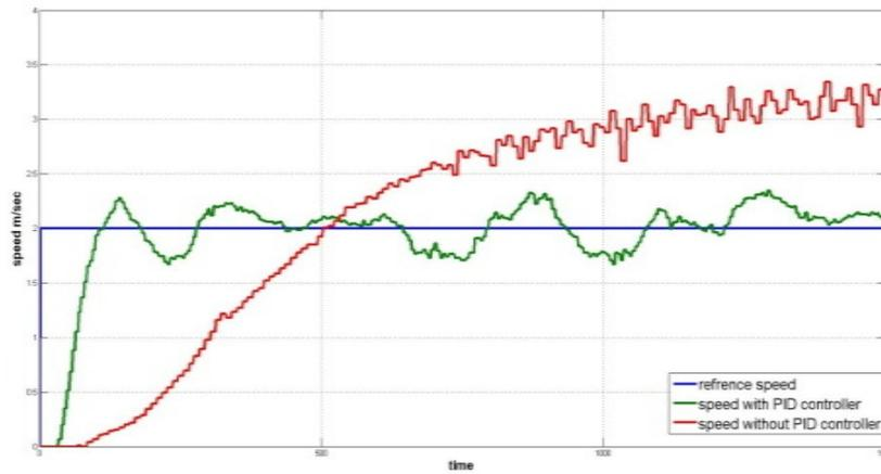
Figure 8 the real system with and without controller
