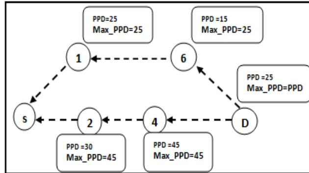
Fig. 4: Route Reply of proposed CLDM-AODV
