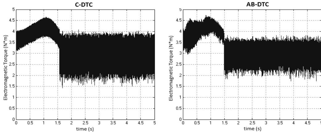
Figure 6. Electromagnetic torque responses at loaded working conditions
