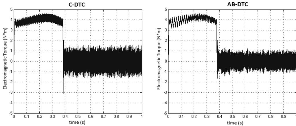
Figure 5. Electromagnetic torque responses at unloaded working conditions
