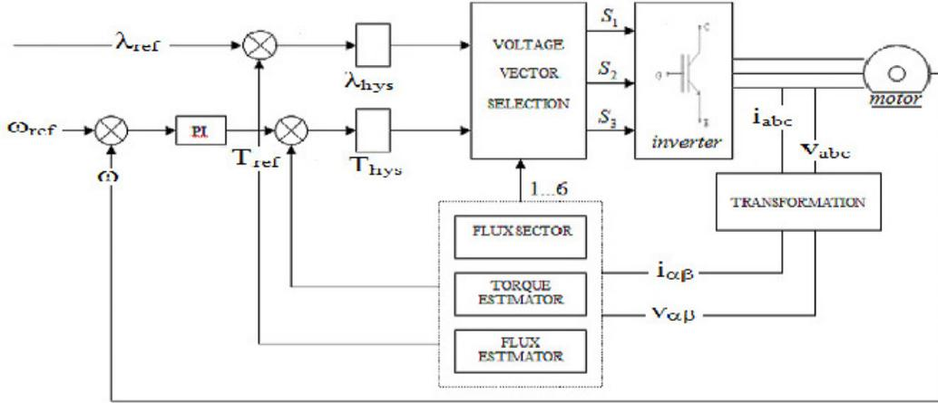
Figure 2. The block diagram of the conventional DTC
