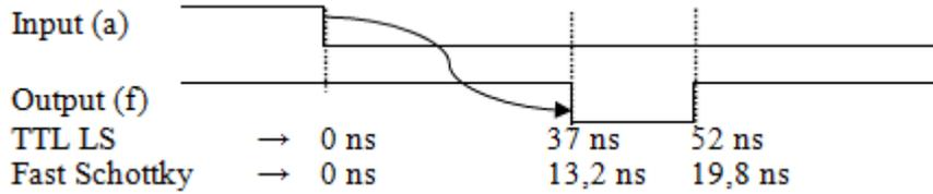
Fig.6. Output waveform for input a transition “1”↓”0”
