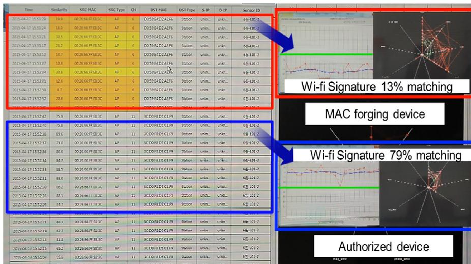
Figure 7. Snapshot of the test platform, it shows the MAC verification process in GUI
