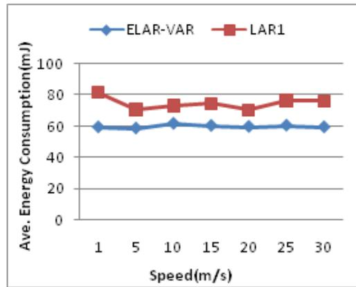
Figure 11. Average Energy Consumption vs. Speed
