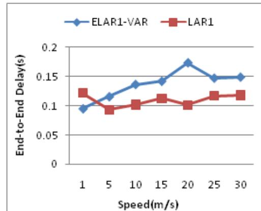
Figure 9. End-to-End Delay vs. Speed
