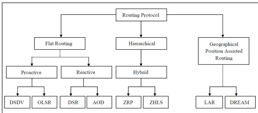
Figure 1. Classification of Routing Protocols
