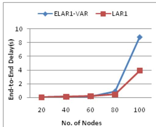
Figure 5. End-to-End Delay vs. No. of Nodes
