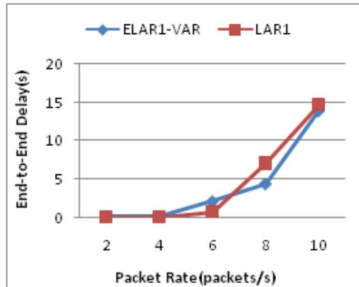
Figure 13. End-to-End Delay vs. Packet Rate
