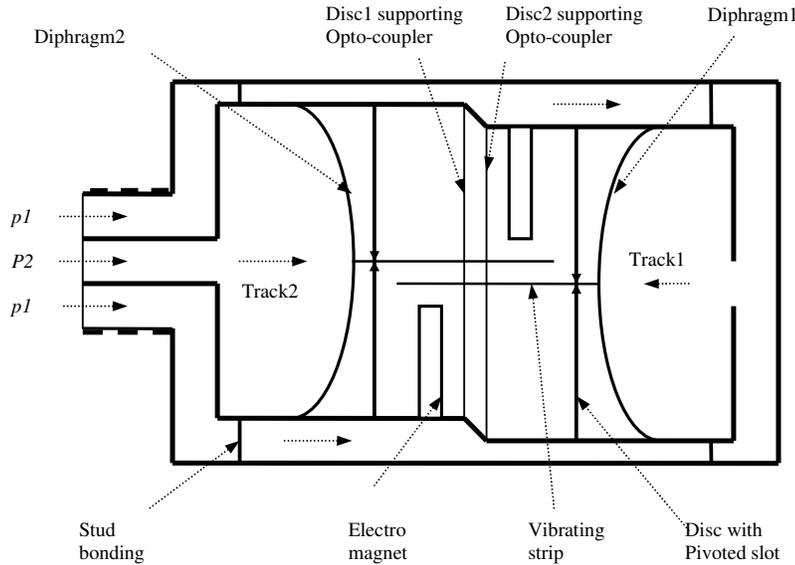
Figure 2. Structure of the differential pressure sensor
