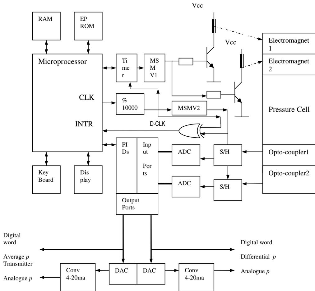
Figure. 4. Simplified schematic of the control schemes and circuits for pressure sensor and transmitter
