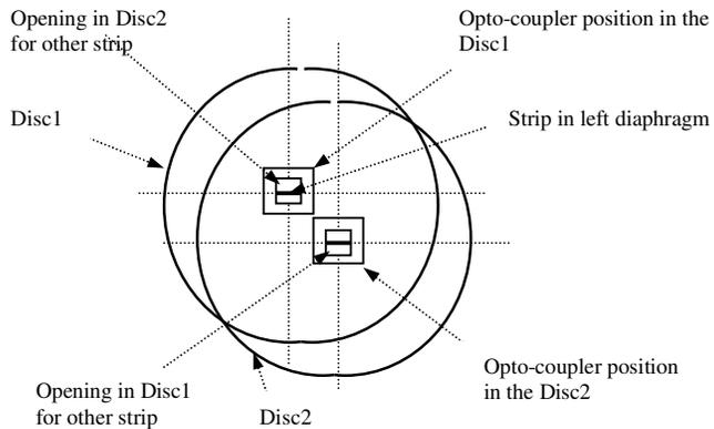
Figure 3. Position of opto-coupler and passage for the strip of other diaphragm
