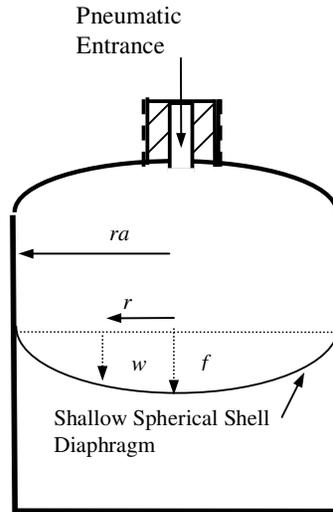
Figure. 1. Schematic of diaphragm based pressure cell
