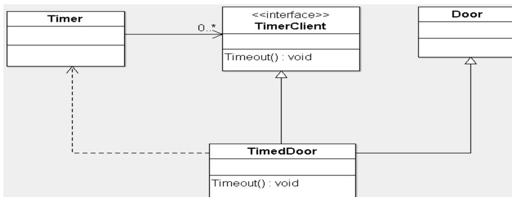
Figure 4. Class Diagram for separation through Multiple Inheritance.
