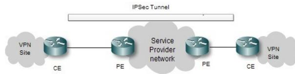
Figure 1. IPsec VPN with CE to CE tunneling.
