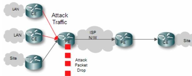
Figure 2. Attack packet dropped at PE router
