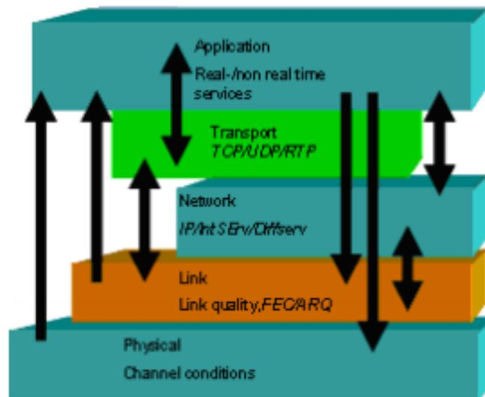
Fig.2. Cross-Layer for wireless protocol stack
