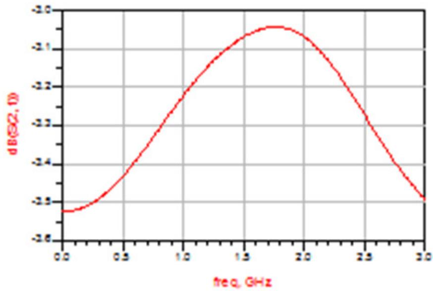
Figure 8: Insertion loss of WPD
