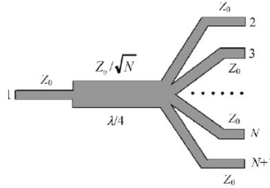
Figure 1: Basic N-way power divider [8,9]
