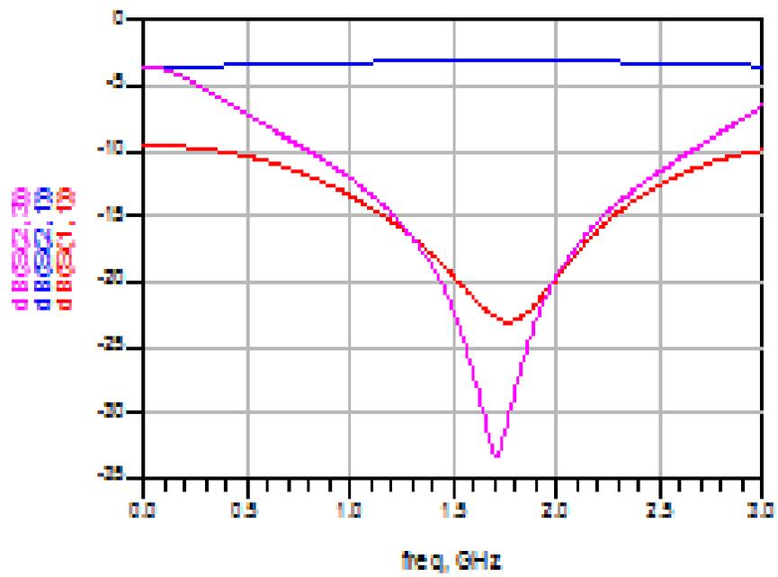
Figure 9: S-parameter simulation of WPD
