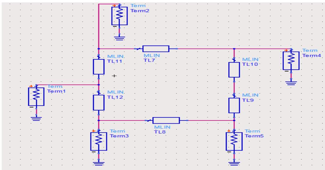
Figure 3: Realization of GPD using ADS®.
