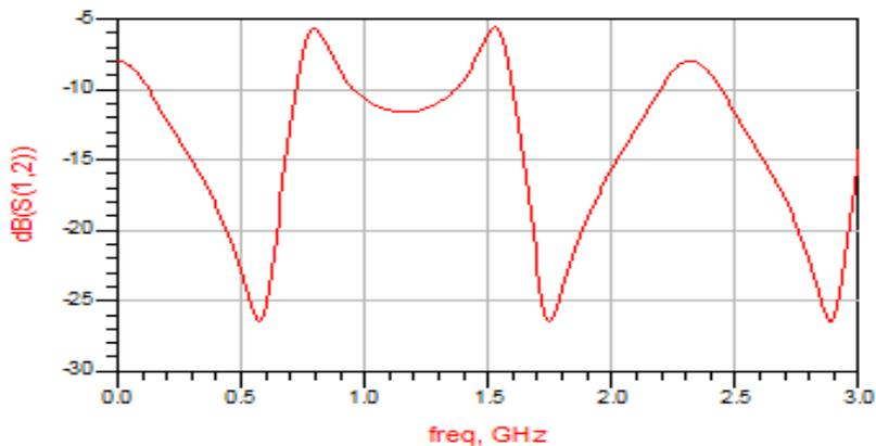
Figure 5: Insertion loss of GPD
