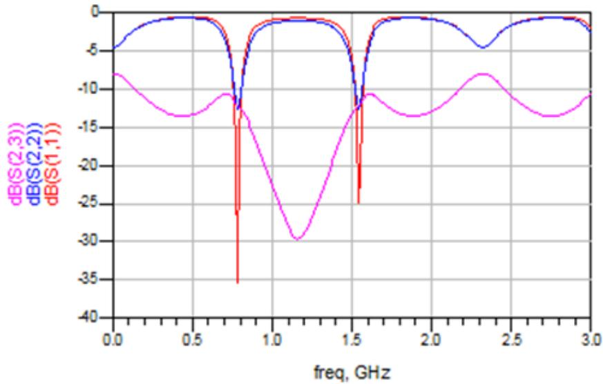
Figure 6: S-parameter simulation of GPD
