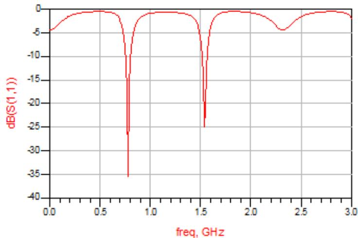
Figure 4: Return loss of GPD
