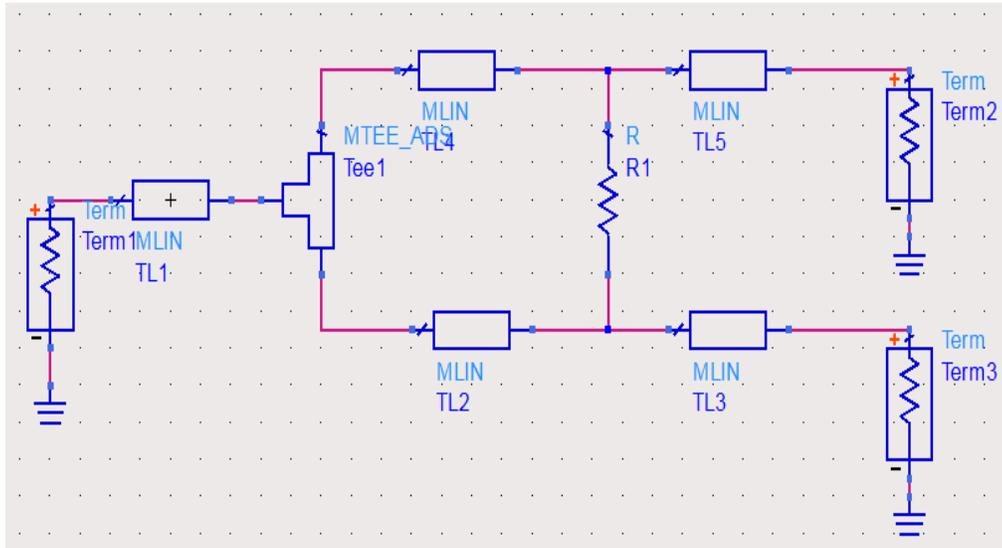
Figure 2: Realization of WPD using ADS®.
