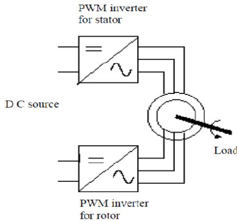
Figure 1. DFIM supplied by two PWM inverters
