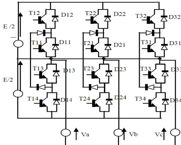
Figure 2. General diagram of a three level PWM inverter
