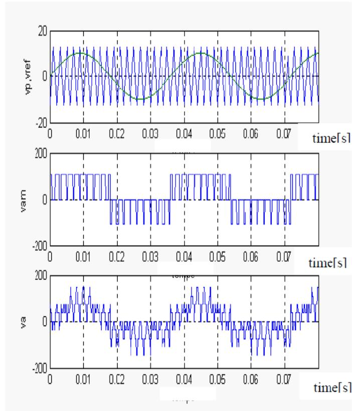
Figure 3 Carrying voltage, simple voltage and phase voltage
