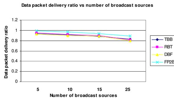
Figure 4: Data packet delivery ratio vs number of broadcast sources
