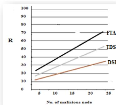
Fig. 7: Comparative graph of Routing Overhead of DSR, T-DSR and FTA with respect to number of malicious nodes
