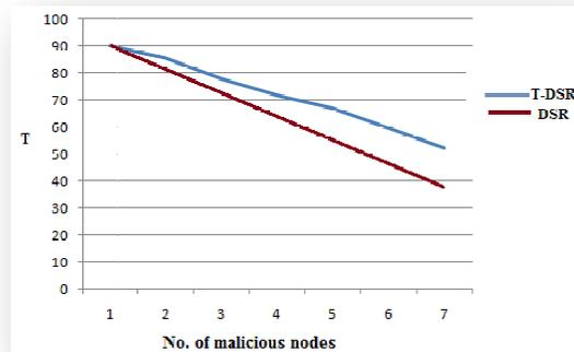
Fig. 2: Comparative graph of Throughput of T-DSR and DSR with respect to number of malicious nodes
