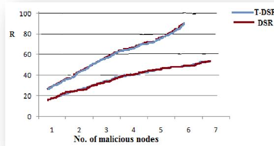
Fig. 3: Comparative graph of Routing overhead of T-DSR and DSR with respect to number of malicious nodes
