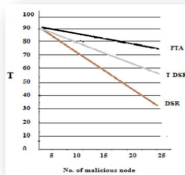
Fig. 6: Comparative graph of Throughput of DSR, T-DSR and FTA with respect to number of malicious nodes
