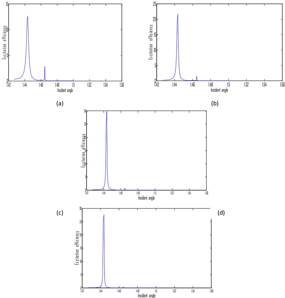
Fig: 5 Variation of excitation efficiency with thickness of superstrate for (a)  $d_2 = 0.3 \mu\text{m}$  (b)  $d_2 = 0.4 \mu\text{m}$  (c)  $d_2 = 0.5 \mu\text{m}$  and (d)  $d_2 = 0.6 \mu\text{m}$
