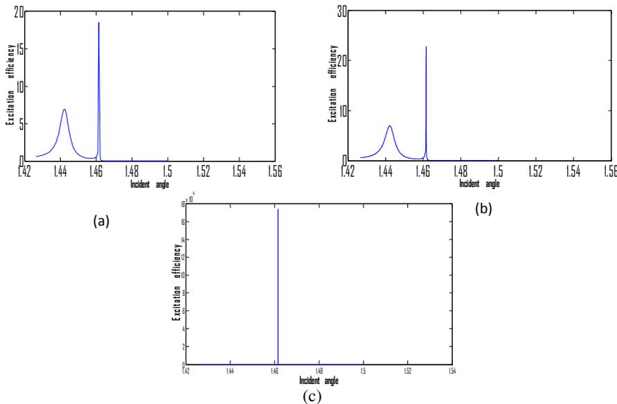
Fig: 4. Variation of excitation efficiency with angle of incidence at first medium for TE mode for resolution of incident angle (a)  $10^{-4}$  (b)  $10^{-5}$  and (c)  $10^{-6}$  with refractive indices for first medium  $n_1 = 1.5$ , second medium  $n_2 = 1.4$ , third medium  $n_3 = 1.5$ , fourth medium  $n_4 = 1.4$  and the thickness of the layers as  $d_1 = 10\mu m$ ,  $d_2 = 0.2\mu m$ ,  $d_3 = 2\mu m$ .
