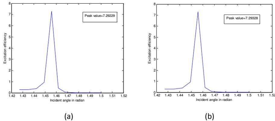
Fig: 6 Excitation efficiency as a function of incident angle for the computation of pure bending loss as (a)  $R=7.2\text{mm}$ ,  $L'=1.2\text{mm}$ , calculated FWHM=0.006980 radian (for positive arc) and (b)  $R=8.5\text{mm}$ ,  $L'=1.3\text{mm}$ , calculated FWHM=0.006916 radian (for positive arc).
