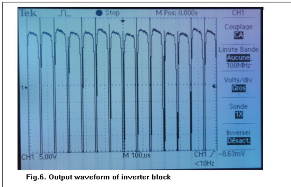
Fig.6. Output waveform of inverter block
