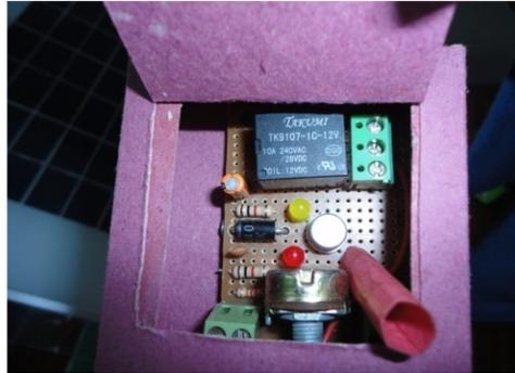
Fig.5. Autonomous intensitycontrolled circuit
