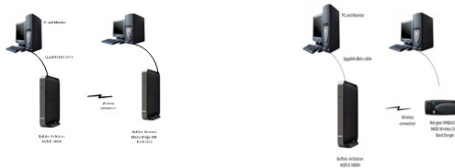
Figure. 2. Buffalo AirStation AC1300/N900 Gigabit Dual Band Wireless Router and Client. (a) With IEEE802.11ac Standard, (b) with Net gear WND3100N600 Wireless Dongle Receiver on IEEE802.11n.
