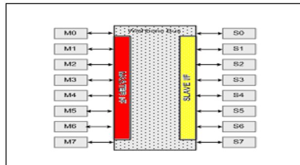
Figure 7. Wishbone core configuration
