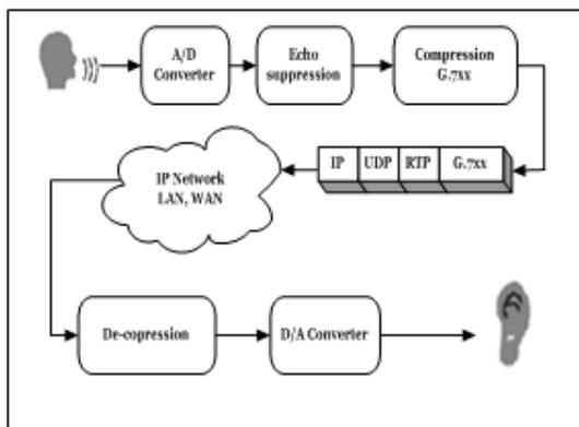
Figure 1. Principle of VoIP
