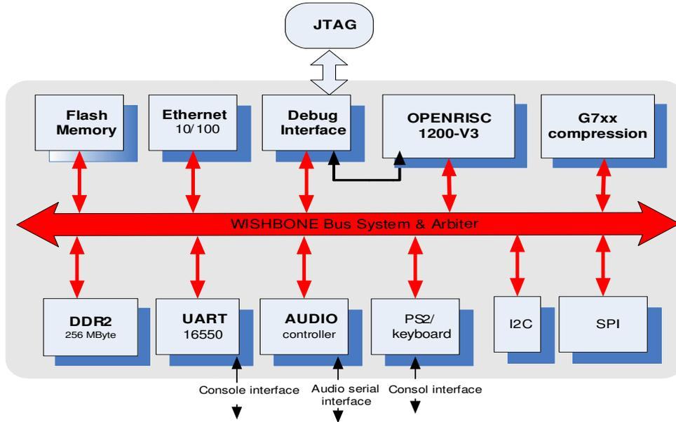
Figure 4 The VOIP Gateway general architecture
