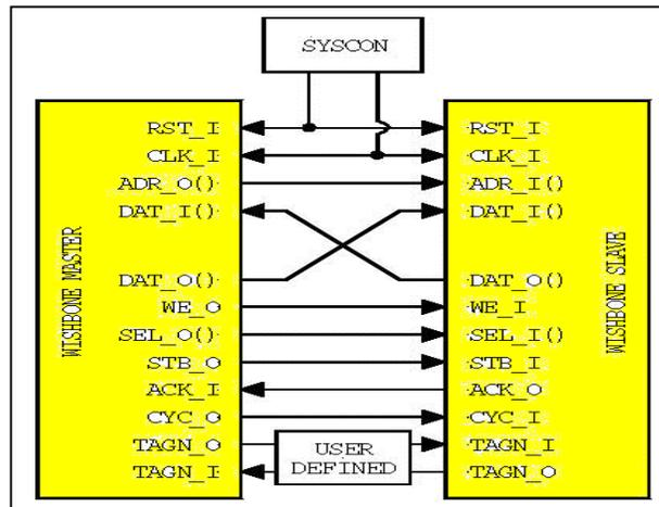
Figure 6. WISHBONE interconnect schema
