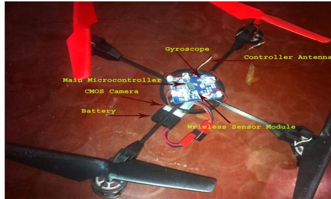
Figure 3. Structure of home-made quadcopters
