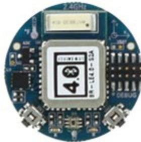
Figure 5. Wireless sensor module
