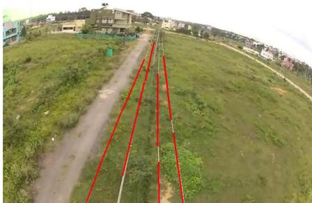
Figure. 1(e): Detected power-lines
