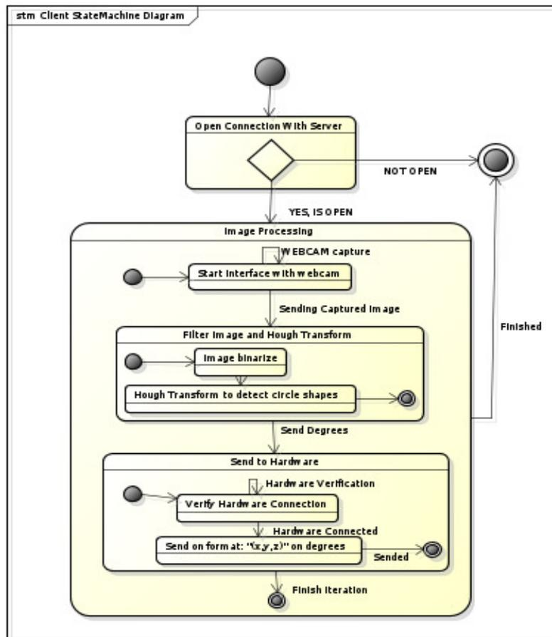
Figure 9. State Machine Diagram Overall Client Program
