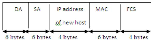
Figure 5. Frame Format of IP\_send message
