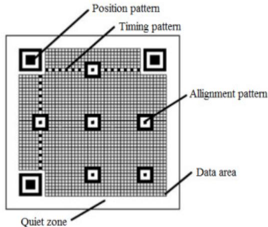
Fig.2. the internal pattern Structure of QR code
