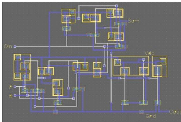
Fig. 8: Proposed adder layout
