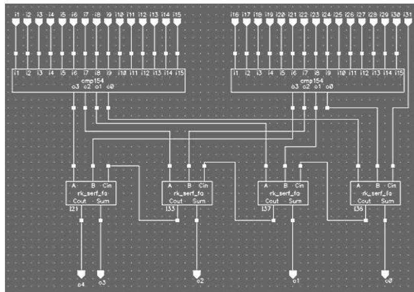
Fig. 7: 31: 5 compressor using lower level compressors
