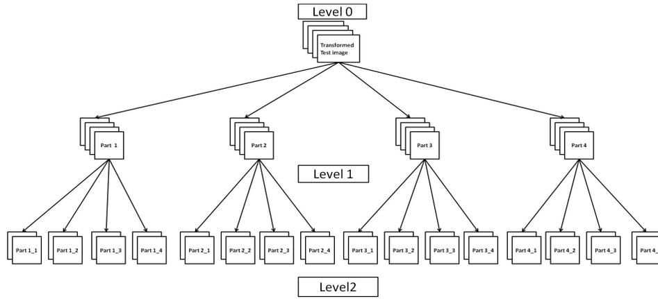
Figure 2: Top down approach of shape matching
