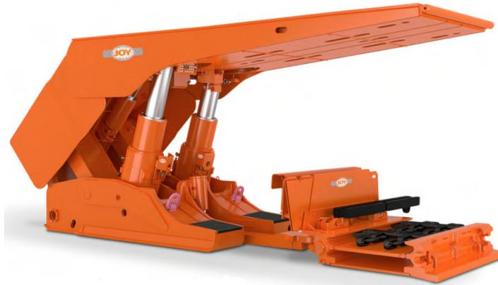
Fig. 3 Single unit of powered roof support (www.joy.com).
