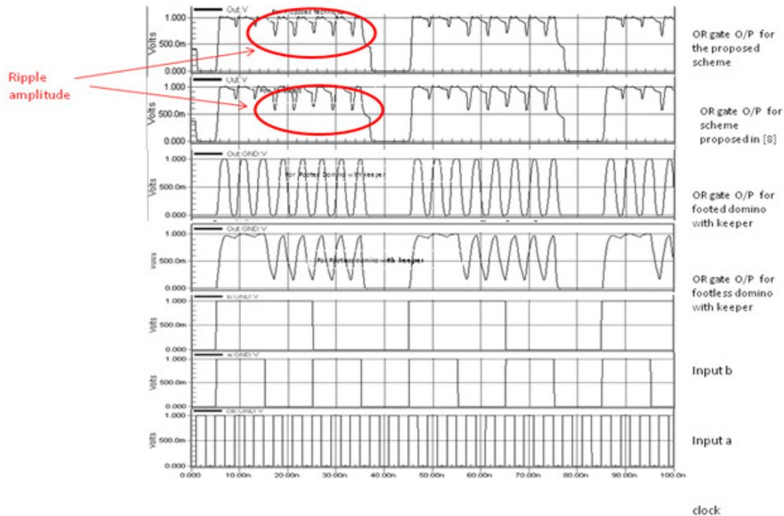
Fig.7 Simulation waveforms of Two input OR gate
