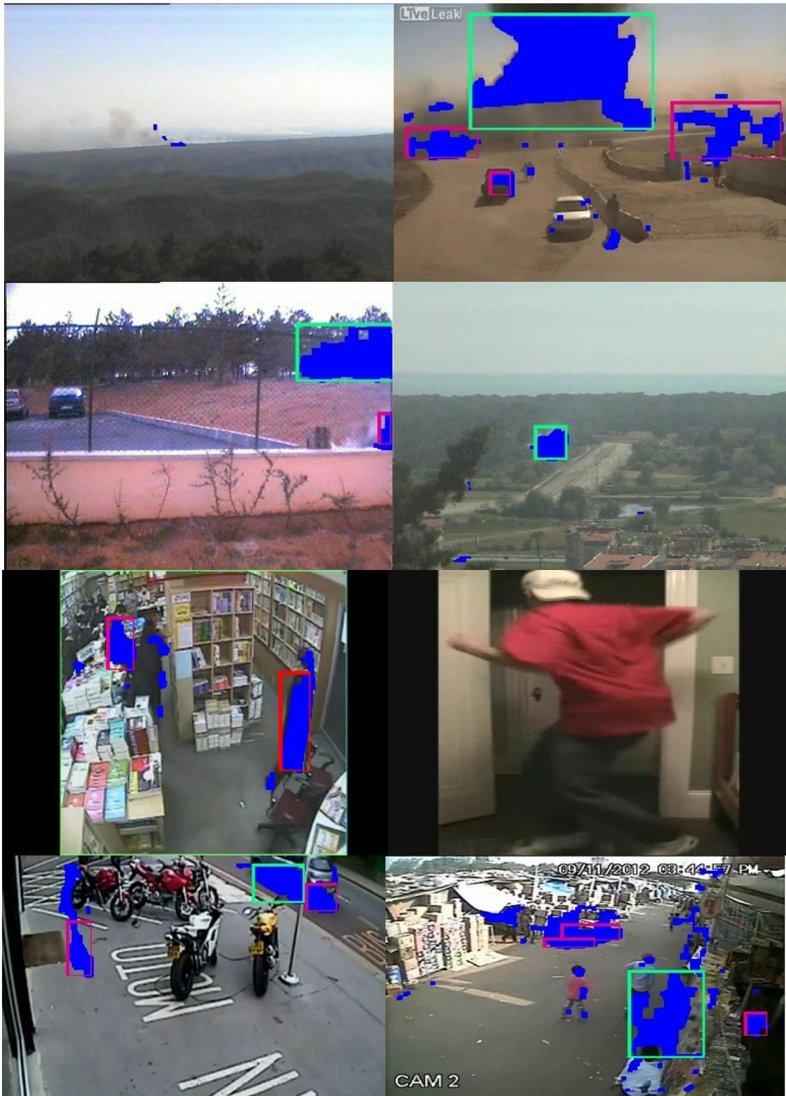
Fig 4. Experimental Result – First 4 Video has smoke, last 4 video do not has smoke
