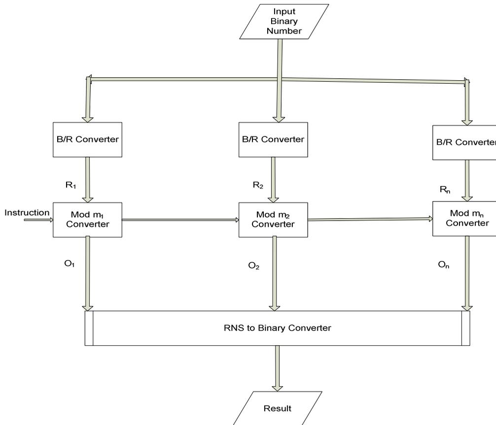
Figure 1. Block diagram of RNS based processing.
