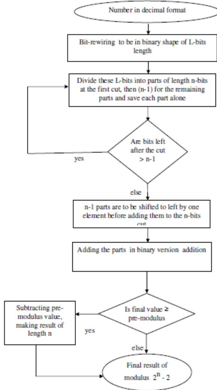
Figure 1. Computing the residue with respect to  $2^n - 2$
