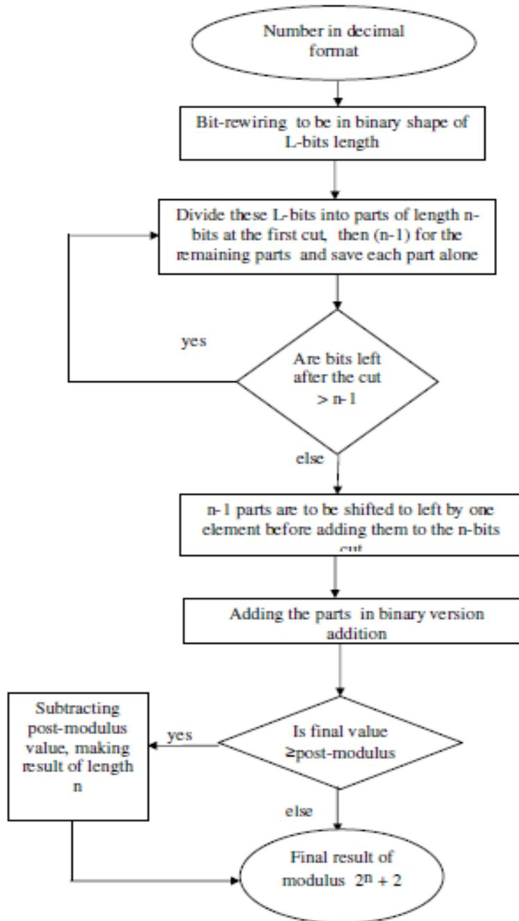
Figure 2. Computing the residue with respect to  $2^n + 2$
