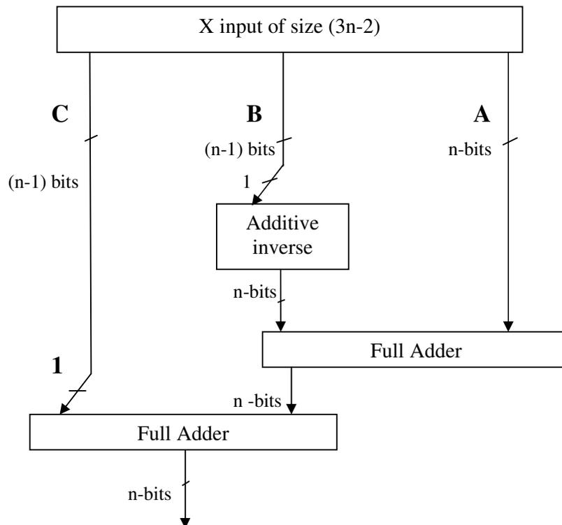
Figure 5. Calculation of Post-modulus ( $2^n + 2$ ).
