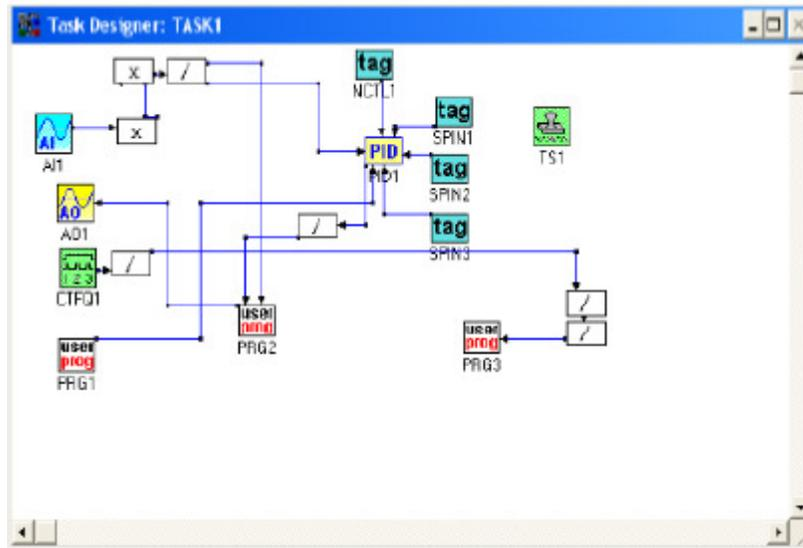
Figure 5. The block diagram of the DAQ-SCADA software
