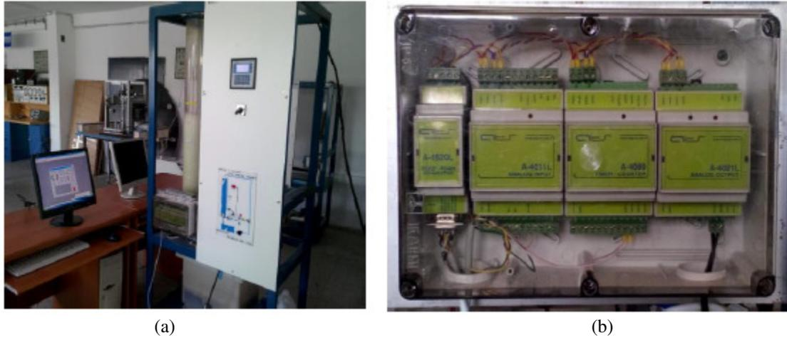
Figure 4. (a) The liquid level control system with computer-controlled and (b) DAQs
