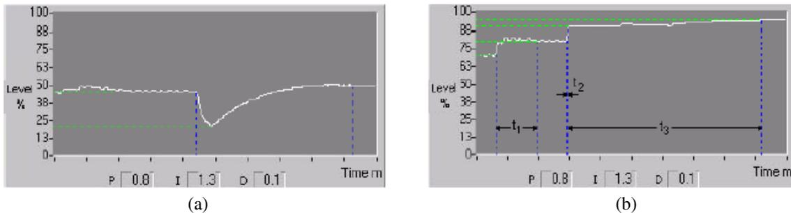
Figure 7. Transient responses for  $K_p = 0.80$ ,  $K_i = 1.27$  and  $K_d = 0.11$ .
