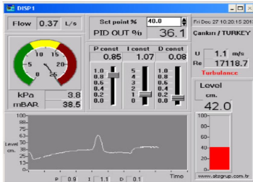
Figure 6. Preview image of the DAQ-SCADA window
