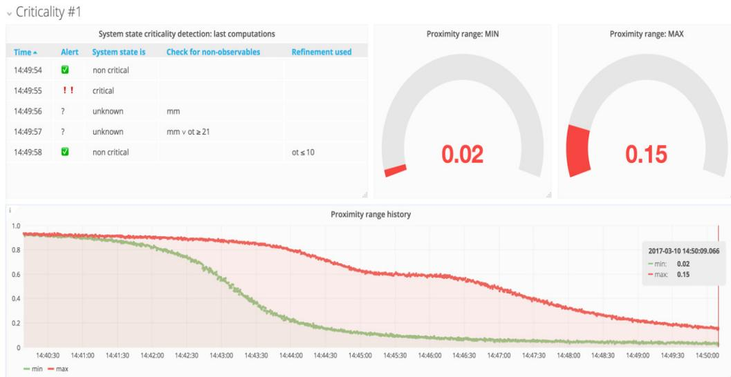
Figure 6. Screenshot of the graphical interface of the monitoring prototype.
