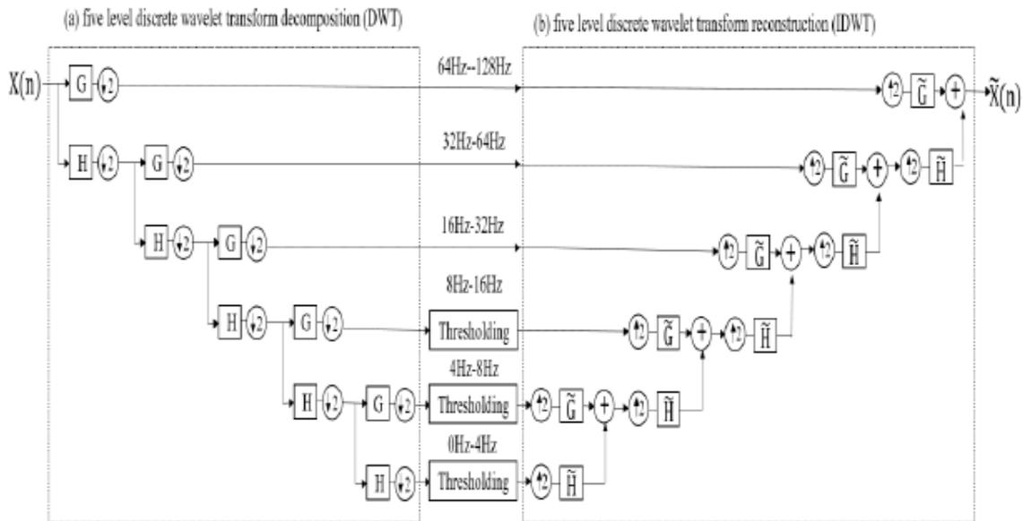
Figure 1. Real-time denoising architecture based on wavelet transform
