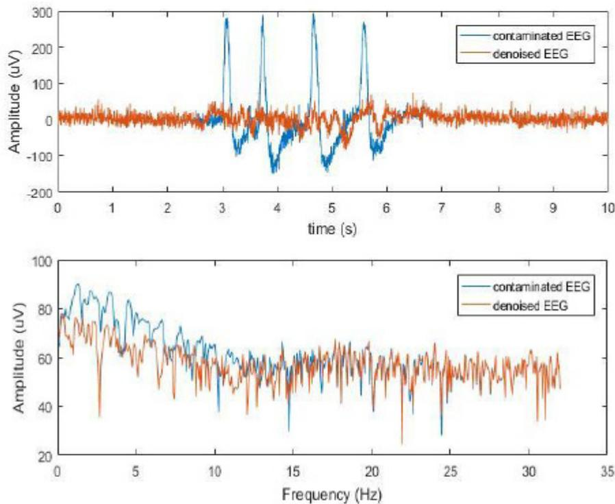
Figure 5. Compare of EEG before and after denoising
