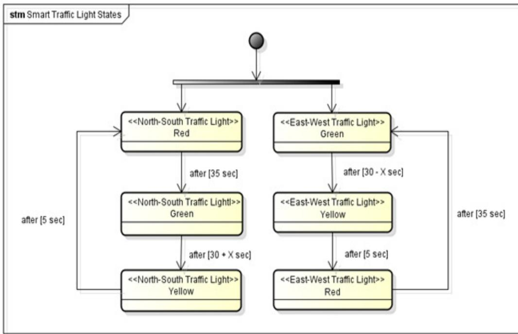
Figure 7. States of Smart Traffic Light System
