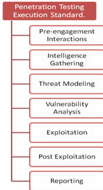
Figure 3: Steps of Penetration Testing Execution Standard
