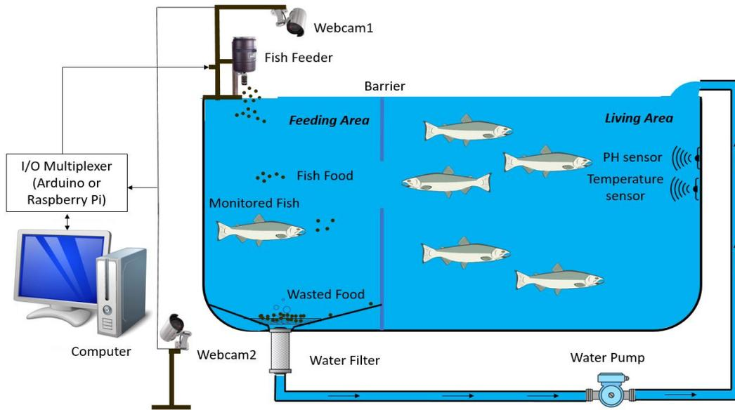
Figure 2. The smart fish feeding system setup
