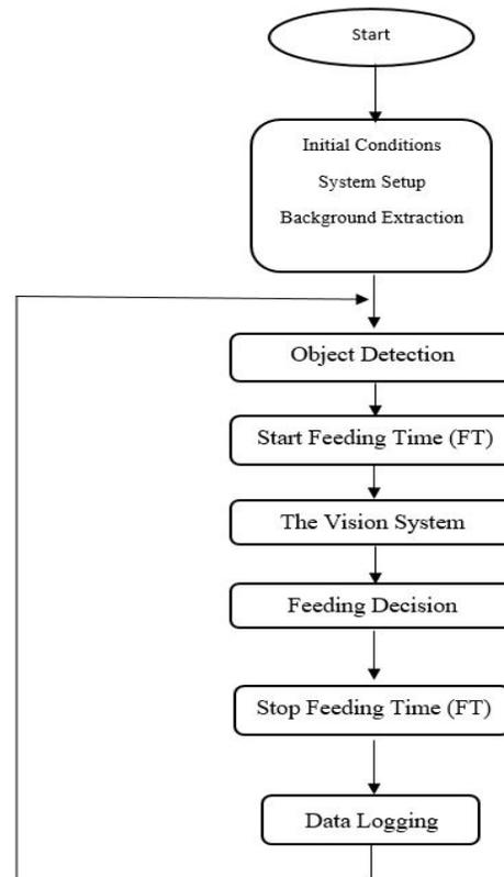
Figure 5. Flowchart of the proposed system algorithm
