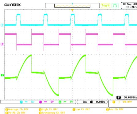
Figure 2.e Test with Firing Angle at 135 degrees
