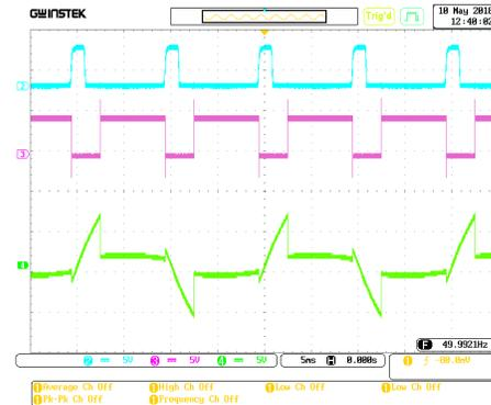
Figure 2.d Test with Firing Angle at 45 degrees
