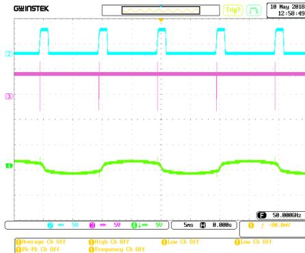
Figure 2.c Test with Firing Angle at 0 degree
