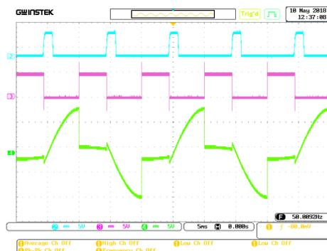
Figure 2.a Triac Functional Testing (90 degrees)
