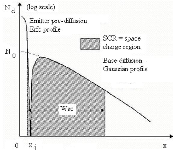
Figure 5. Base-emitter junction doping profile and space charge region (SCR) of a bipolar transistor with diffused base
