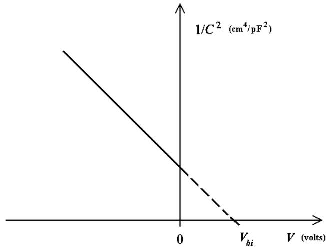
Figure 3.  $1/C^2$  plot of the barrier capacitance used to determine the background concentration  $N_B$  and built-in potential  $V_{bi}$  of a semiconductor junction
