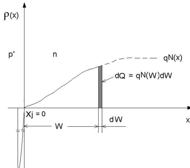
Figure 2. The depletion approximation for the charge distribution in an asymmetric  $p^+n$  junction
