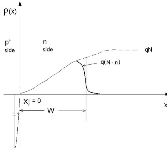
Figure 4. The real case of an asymmetric p<sup>+</sup>n junction charge distribution
