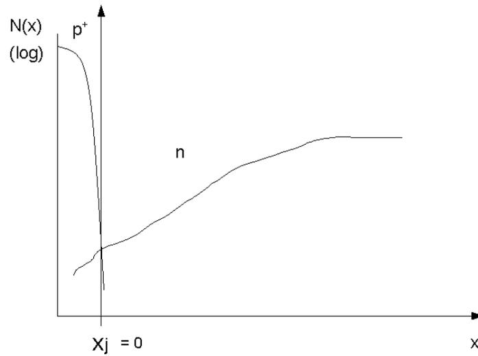
Figure 1. The concentrations of impurities in a  $p^+n$  junction (asymmetric type)
